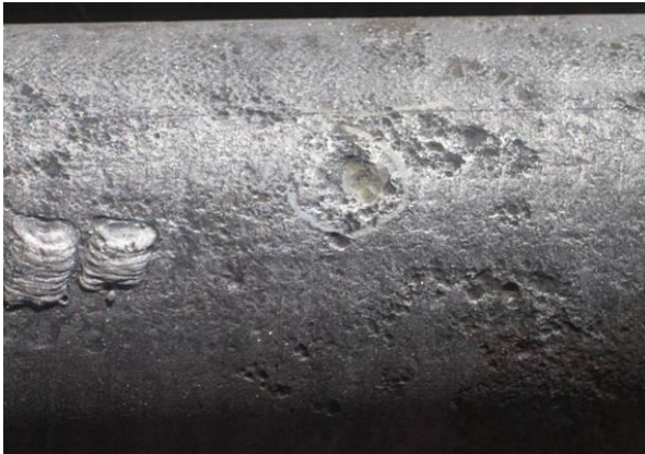
Corrosion pitting, welding defects
